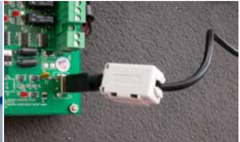
Folding core on the USB cable to the USB IO 1 or 2 x through the core
